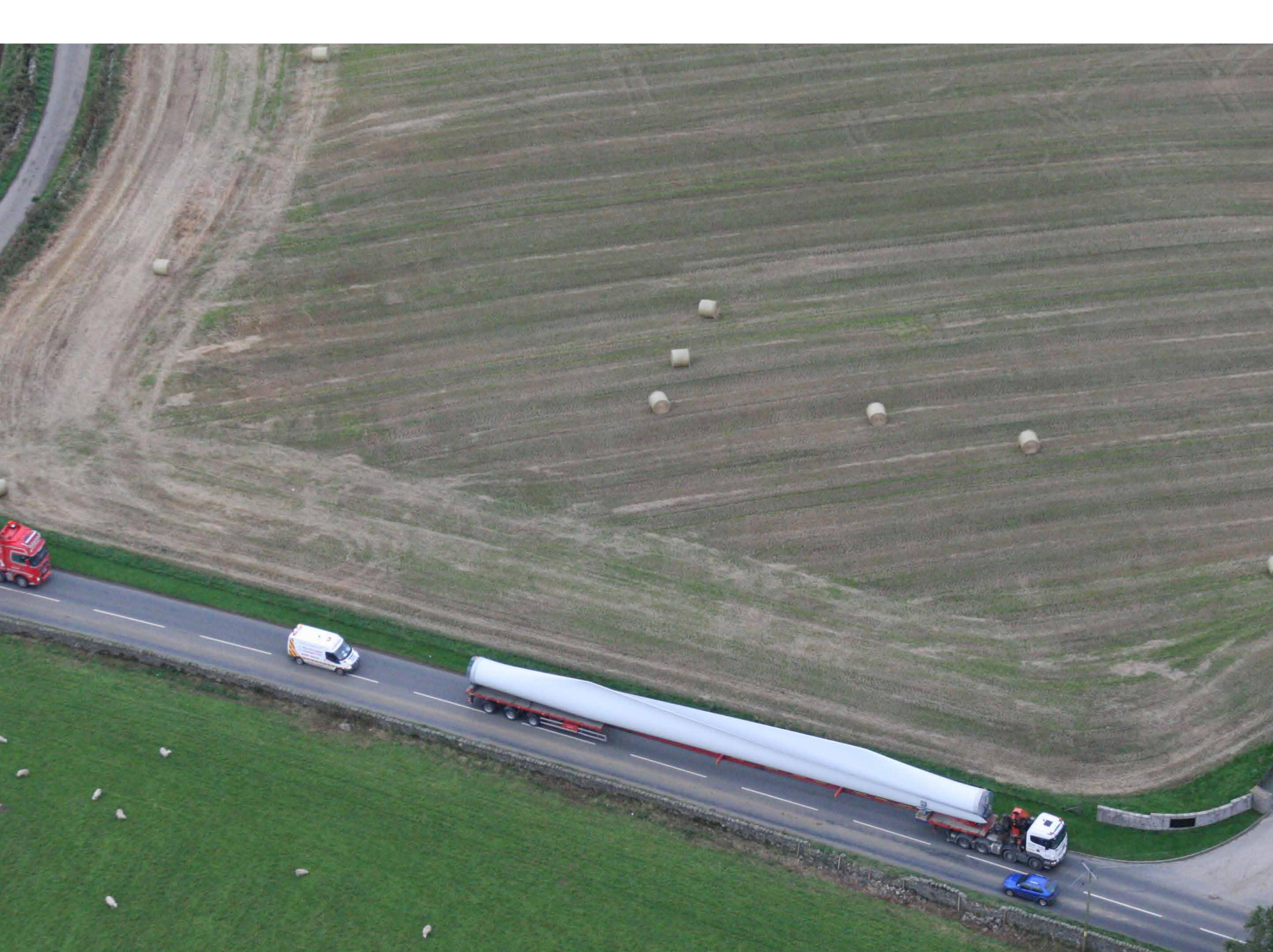
Blade delivery at Hill of Towie Wind Farm, Moray, Scotland | Photo: RES / For illustrative purposes only Turbines: Siemens, 2.3 MW, height to tip of 100 metres
